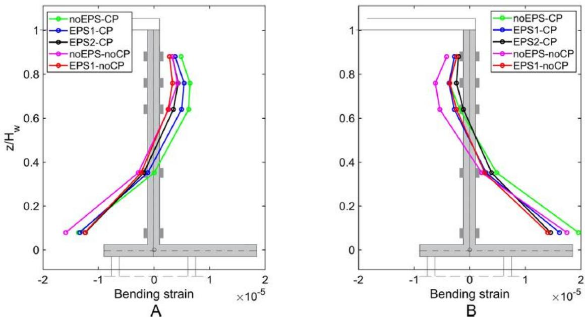
Figure 3: Indicative results of the maximum (left) and minimum (right) bending strain on the abutment wall for different EPS configurations measured as part of the H2020 project SERA in EQUALS Lab [5]
