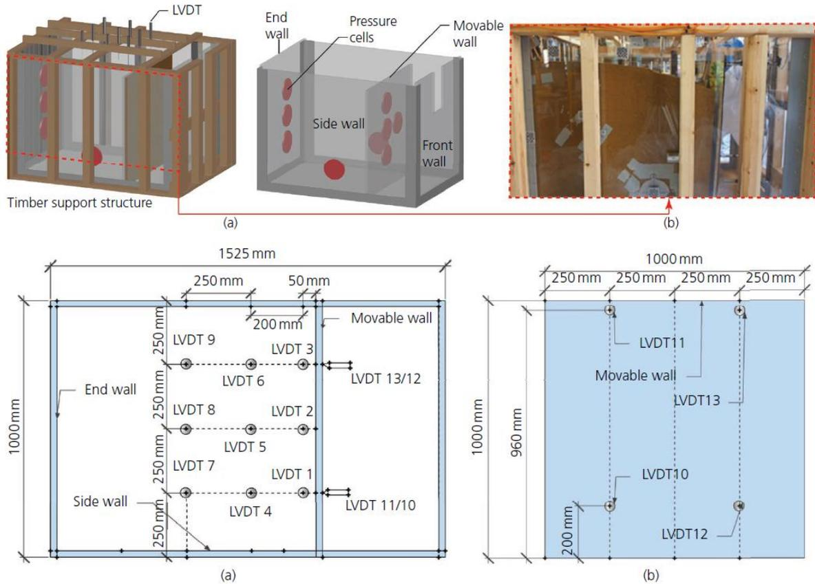
Figure 1: Annotated three-dimensional diagram of the test box; (b) test box filled with LBS (top). Layout of the LVDTs: (a) plan view of the test box; (b) front view of the movable wall (bottom)[6]
