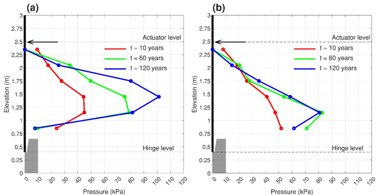
Figure 6: (a) Passive and (b) active pressures along the wall for an equivalent period of 10, 60 and 120 years.
