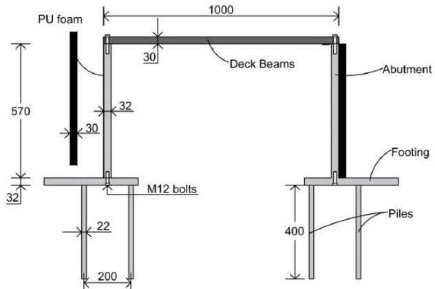
Figure 2: Shear stack configuration containing the scaled integral bridge tested on the 3m x 3m shaking table of the EQUALS Laboratory at the University of Bristol (left) Section of the bridge model (right). All dimensions are in mm. The specific rig was part of the H2020 project SERA [5,7]
