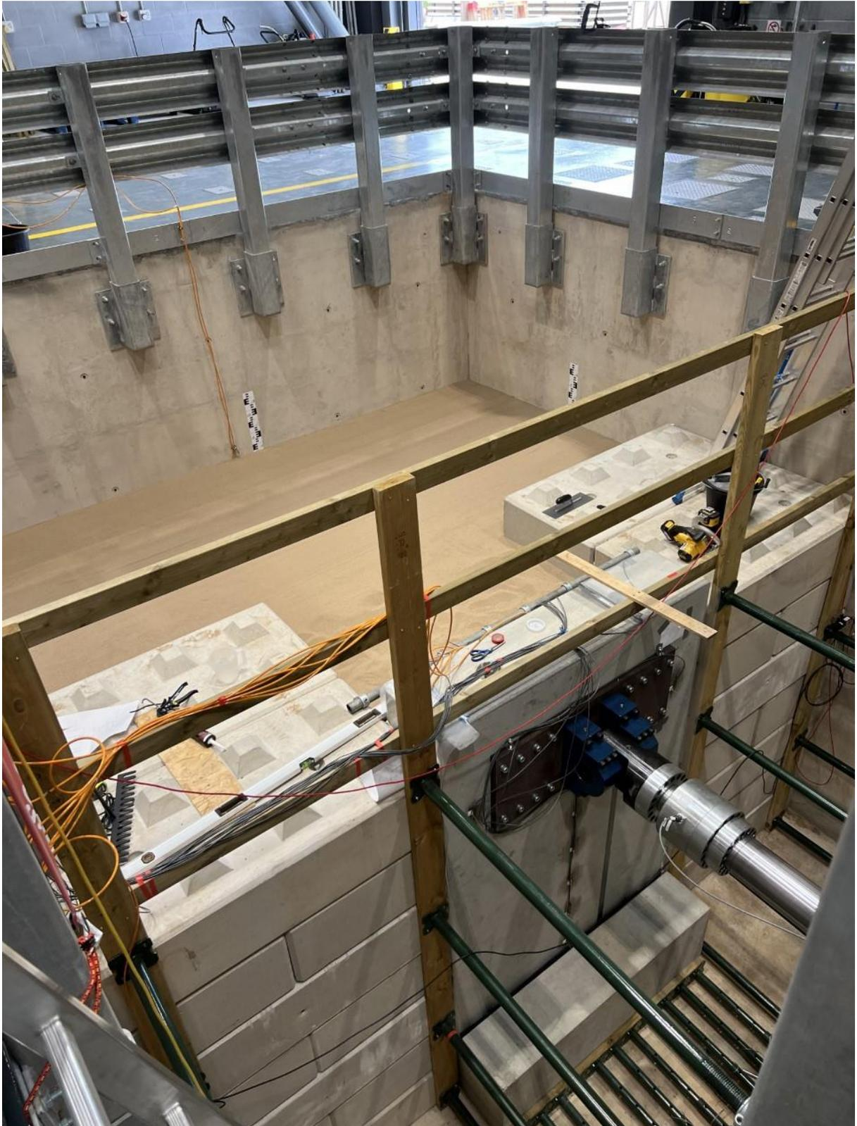
Figure 4: Overview of the SoFSI Soil Pit and the test configuration, including the abutment (flap wall), the hinged base and the loading configuration.
